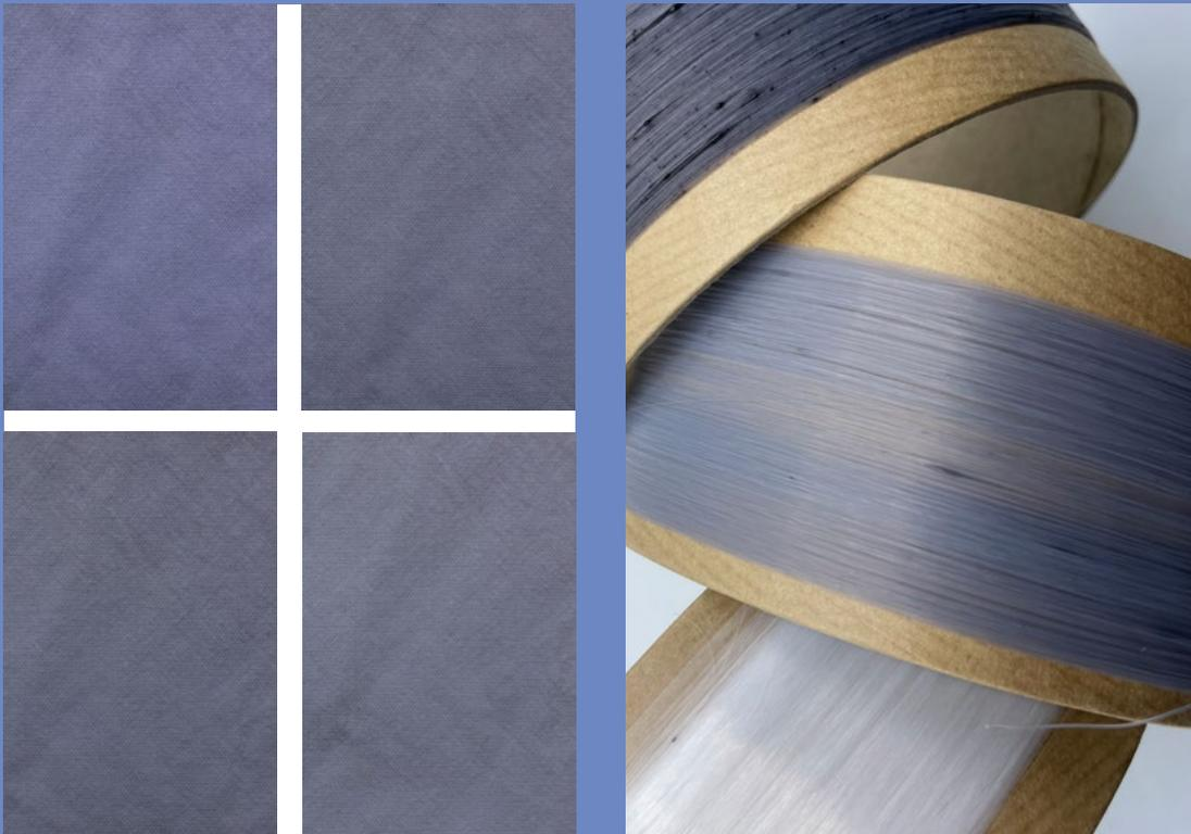
Figure 7 Materials samples of textiles coloured with microbial colourants, showing the effect of exposure to light (left) (DIA 18) and PP melt spun with violacein (right) (DIA 40).
