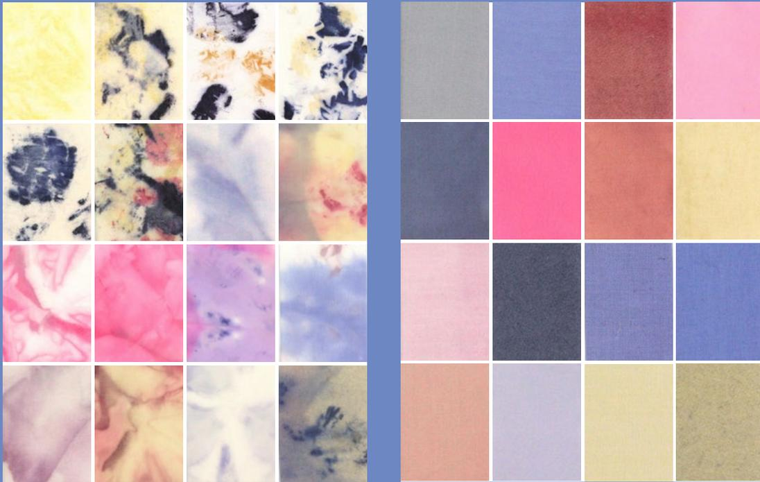
Figure 6 Materials samples of textiles coloured with microbial colourants (DIA 5).
